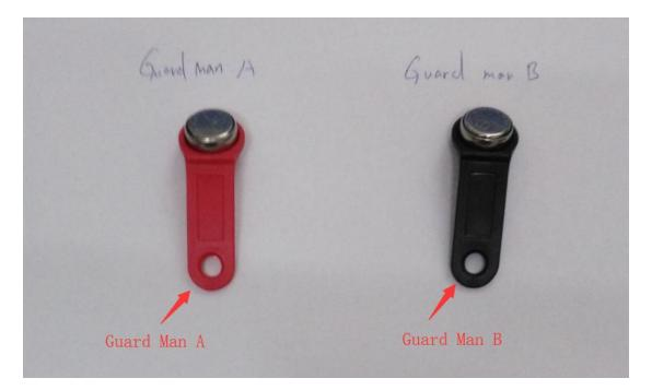
then for example when john go to patrol, using the wand read his own person button firstly, then bring the wand reader(NOT bring the red or black tag to read) with him and go out to read different location check point(read by the wand reader, not by the person button), the system will know these patrol records below to John.
